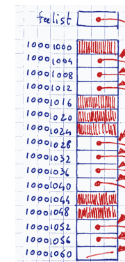
Figure: Think of the binary representation of pointers to heap objects: here any pointer will end with 00 (because addresses in radix 10 are divisible by 4).
