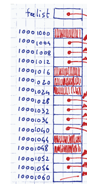
Figure: A 16-word heap with a free list : each unused word in the heap points to the next one. Red words belong to alive objects.
